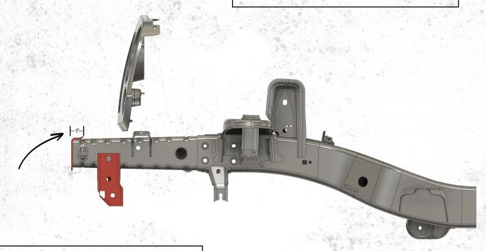
IF YOU HAVE TROUBLE REMOVING THE FRAME BRACKETS, YOU CAN CUT 1" OFF YOUR FRAME END.
