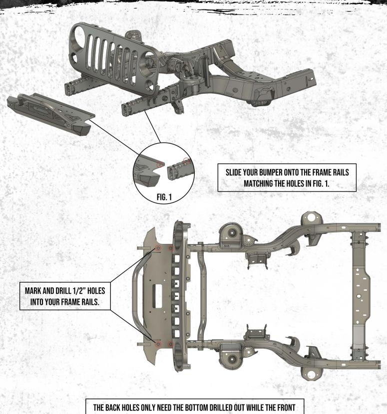
HOLES WILL NEED TO BE DRILLED ALL OF THE WAY THROUGH.
